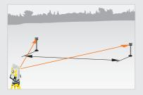
Missing Line Measurement Determine the distance, grade, azimuth and height difference between any two points. Determining ties is a breeze.
